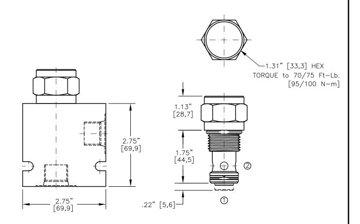
NOTE: CAVITY BOTTOM HOLE MUST ALLOW FOR POPPET EXTENSION (.750" DIA.) FOR ALUMINUM OR STEEL VALVE HOUSING CONFIGURATIONS SEE PAGE 0-013.1
